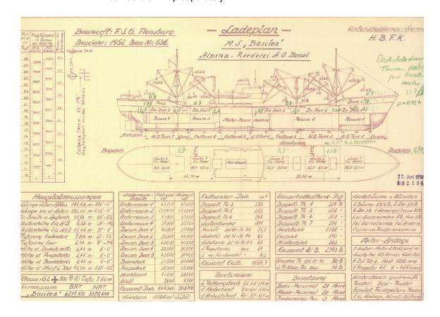
In this loading plan (capacity plan) the "deadweight scale" is located in the left, upper corner.
